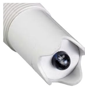
Figure 5 Low temperature (LT) glass with notched body
